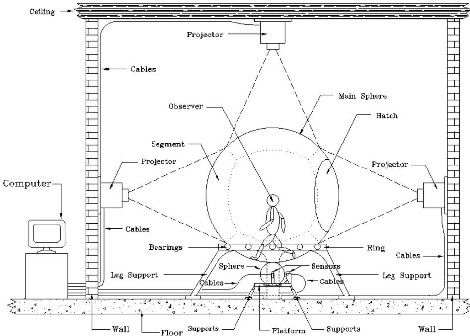
**Figure 1.** Schematic of the Cybersphere.
