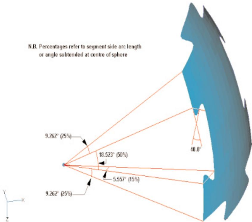
**Figure 2.** Interlocking segments of the Cybersphere.
