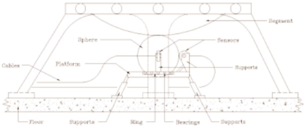
**Figure 3.** Secondary rotating sensing sphere.
